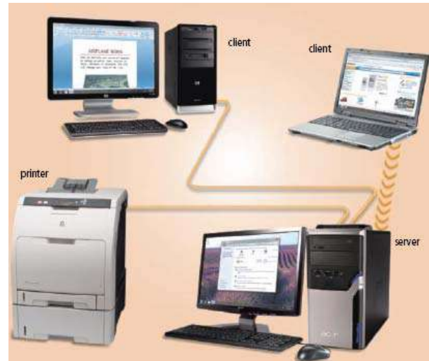
Figure 1-6 A server manages the resources on a network, and clients access the resources on the server. This network enables three separate computers to share the same printer, one wirelessly.
