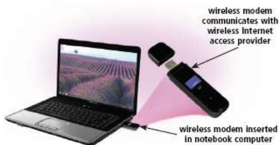
Figure 9-28 Wireless modems allow users to access the Internet wirelessly using the cell phone network.
