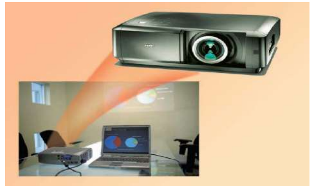
Figure 6-29 A data projector projects an image from a computer screen on a larger screen so that an audience easily can see the image.
