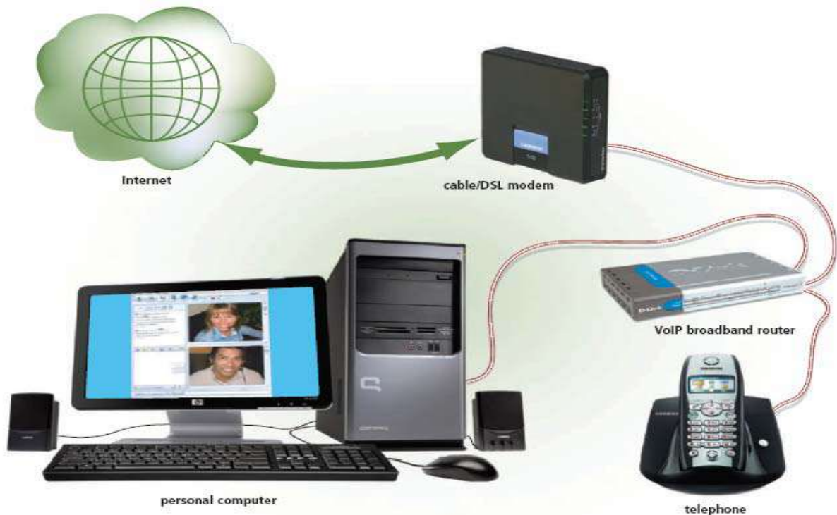
Figure 2-31 One type of equipment configuration for a user making a call via VoIP.
