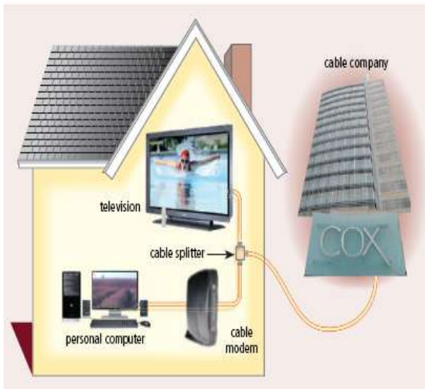
Figure 9-27 A typical cable modem installation.
