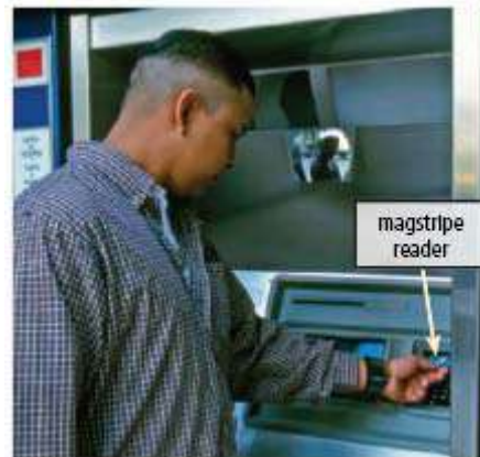
Figure 5-41 An ATM is a self-service banking terminal that allows customers to access their bank accounts.
