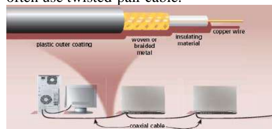
Figure 9-37 On a coaxial cable, data travels through a copper wire. This illustration shows computers networked together with coaxial cable.
