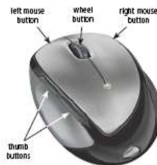
Figure 5-6 This mouse uses a laser to detect movement of the mouse. It also includes buttons you push with your thumb that enable forward and backward navigation through Web pages.
