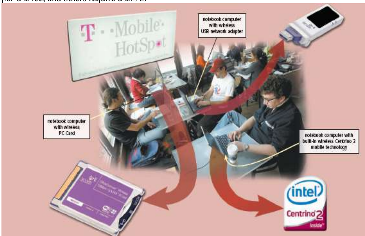
Figure 9-4 Mobile users in this hot spot access the Internet through their notebook computers. One computer uses a wireless USB network adapter; another uses a wireless PC Card. Others have Intel's built-in wireless Centrino 2 mobile technology.
