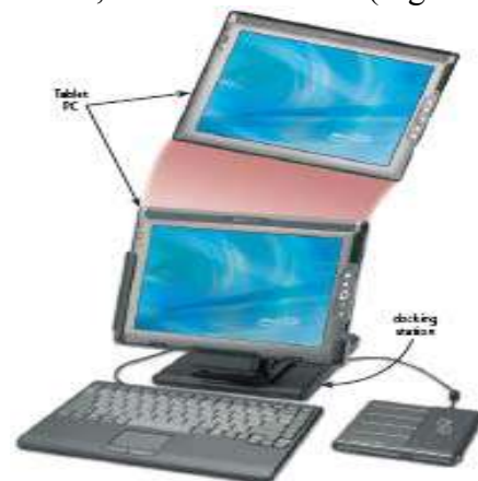
Figure 4-35 To use a slate Tablet PC while working at a desk, insert the Tablet PC in a docking station. Devices such as a keyboard and an optical disc drive can be plugged in the docking station.
