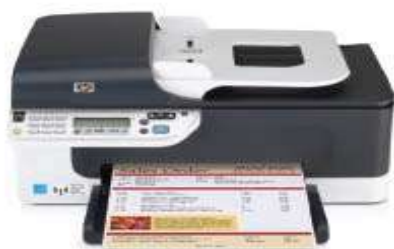
Figure 6-20 This multifunction peripheral is a color printer, scanner, copy machine, and fax machine.
