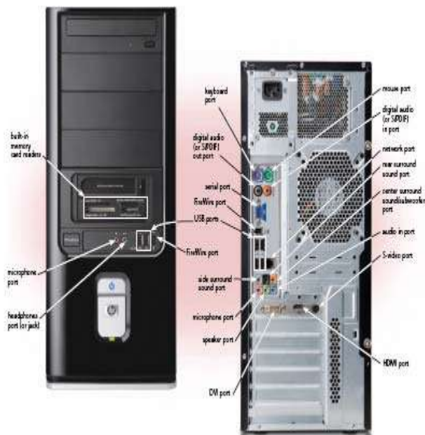
Figure 4-29 A system unit on a desktop personal computer has many ports on its front and back.
