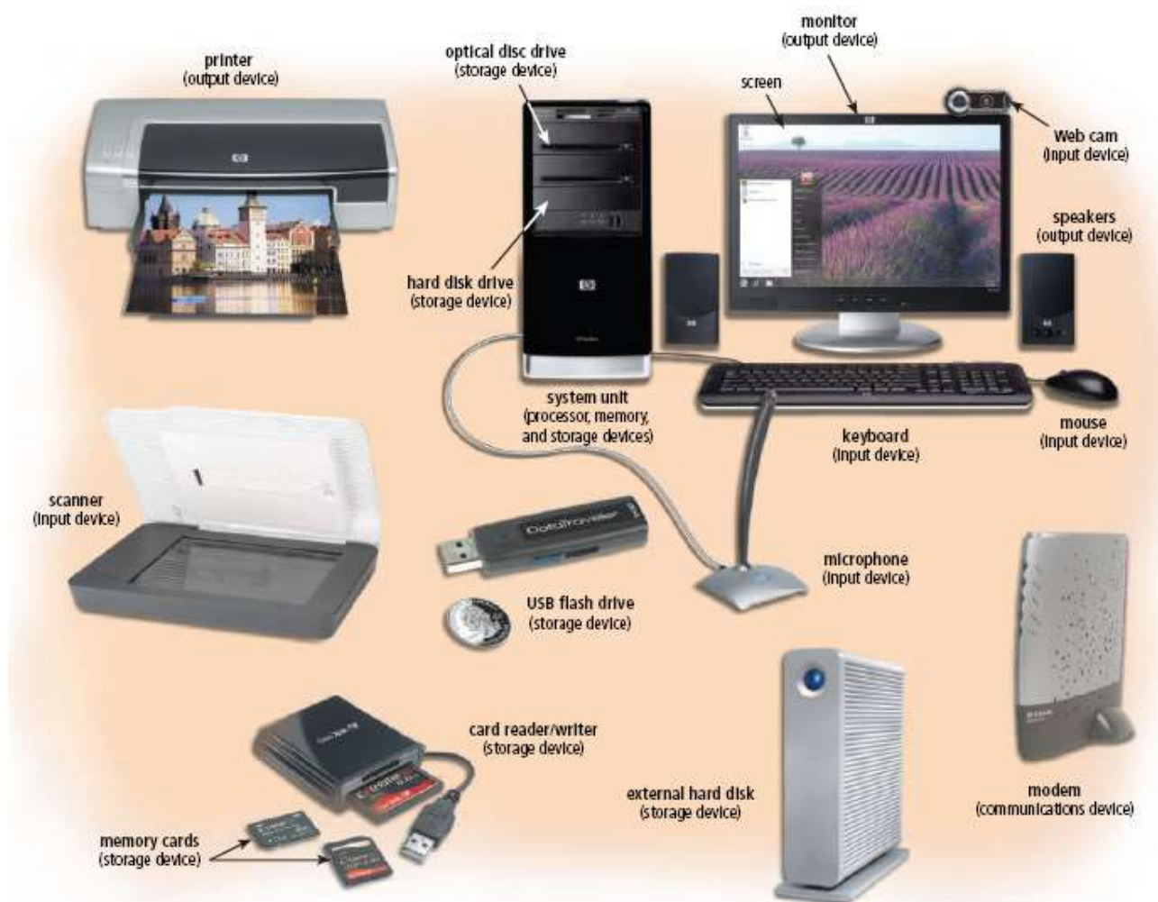
Figure 1-3 Common computer hardware components include a keyboard, mouse, microphone, scanner, Web cam, printer, monitor, speakers, system unit, hard disk drive, external hard disk, optical disc drive(s), USB flash drive, card reader/writer, memory cards, and modem.
