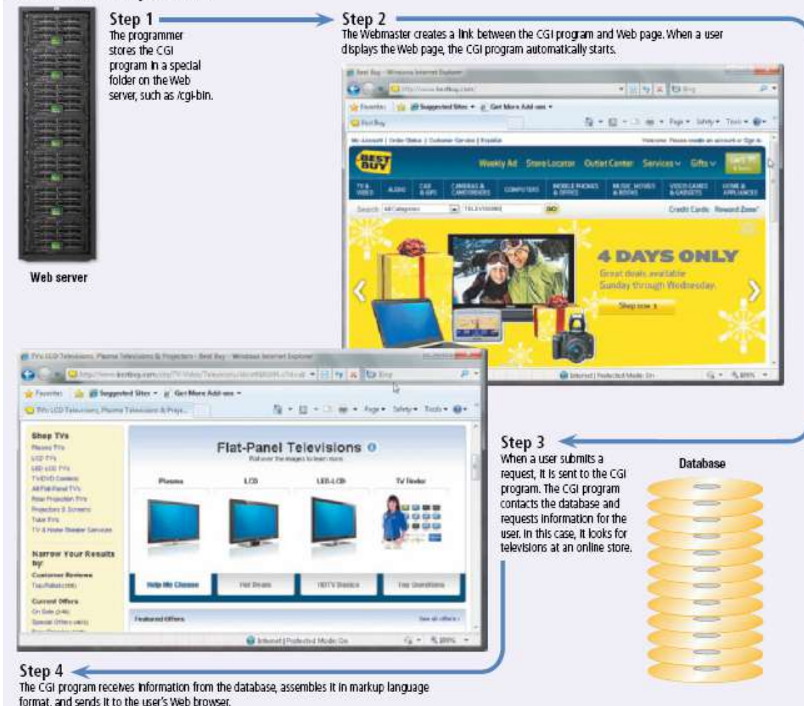
Figure 10-19 This figure shows how a CGI script works.
