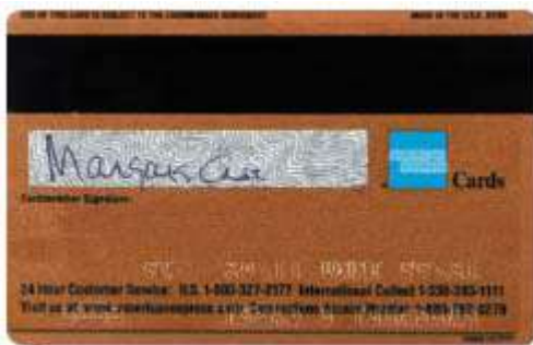
Figure 5-34 A magnetic stripe card reader reads information encoded on the stripe on the back of your credit card.
