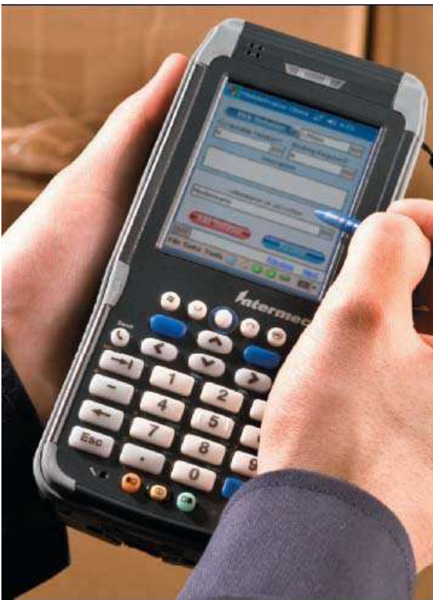
Figure 1-21 This handheld computer is a lightweight computer that enables delivery people to obtain and record information about their deliveries.
