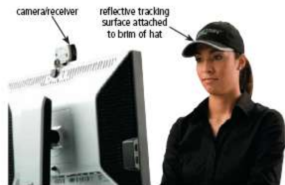
Figure 5-45 A camera/receiver mounted on the monitor tracks the position of the head-mounted pointer, which is reflective material that this user is wearing on the brim of her hat. As the user moves her head, the pointer on the screen also moves.
