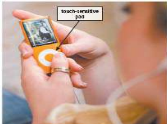
Figure 5-15 You use your thumb to rotate or press buttons on a Click Wheel.
