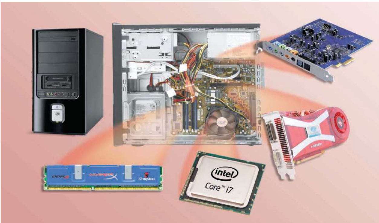
Figure 4-2 The system unit on a typical personal computer consists of numerous electronic components, some of which are shown in this figure. The sound card and video card are two types of adapter cards.
