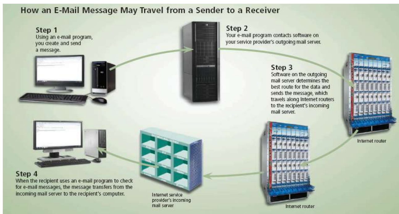
Figure 2-27 This figure shows how an e-mail message may travel from a sender to a receiver.
