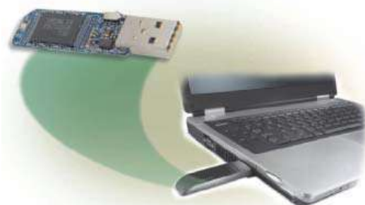
Figure 7-21 A close-up of the flash memory and circuitry inside a USB flash drive.
