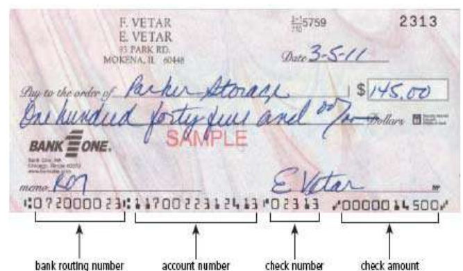
Figure 5-35 The MICR characters preprinted on the check represent the bank routing number, the customer account number, and the check number. The amount of the check in the lower-right corner is added after the check is cashed.
