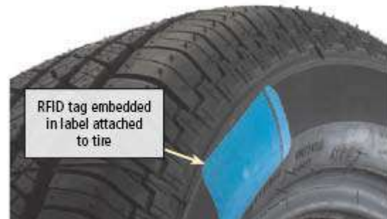
Figure 5-33 RFID readers read information stored on an RFID tag and then communicate this information to computers, which instantaneously compute payments and update inventory records. In this example, the RFID tag is embedded in a label attached to the tire.
