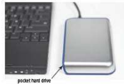
Figure 7-16 Users easily can transport data from one computer to another with a pocket hard drive.
