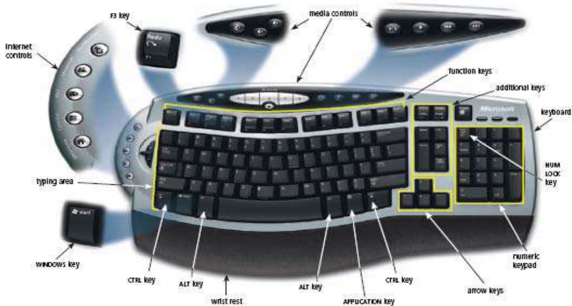
Figure 5-2 On a desktop computer keyboard, you type using keys in the typing area and on the numeric keypad.
