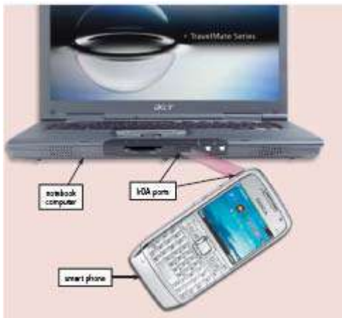
Figure 4-34 Many devices communicate wirelessly with desktop or notebook computers through IrDA ports.
