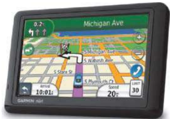
Figure 1-42 This handheld navigation device gives users turn-by-turn voice-prompted directions to a destination.
