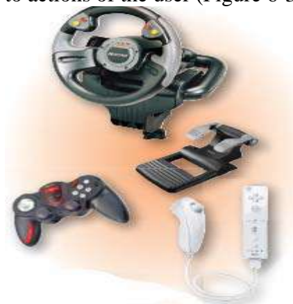
Figure 6-31 Gaming devices often provide force feedback, giving the user a realistic experience.
