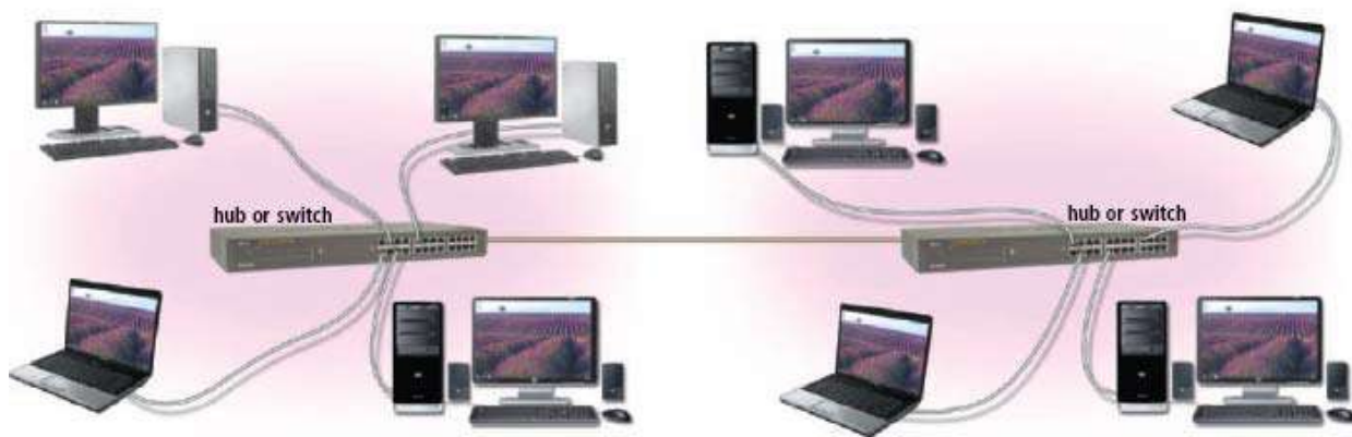
Figure 9-32 A hub or switch is a central point that connects several devices in a network together.
