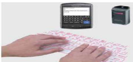
Figure 5-18 The characters you type on this full-sized optical key board appear on your smart phone.
