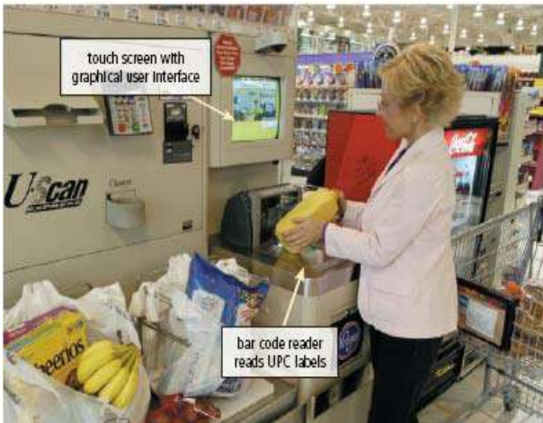
Figure 5-40 Many grocery stores offer self-serve checkouts, where the consumers themselves use the POS terminals to scan purchases, scan their store saver card and coupons, and then pay for the goods.
