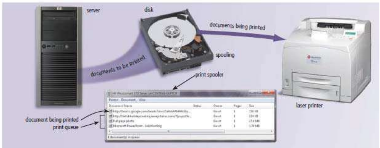
Figure 8-9 Spooling increases both processor and printer efficiency by placing documents to be printed in a buffer on disk before they are printed. This figure illustrates three documents in the queue with one document printing.
