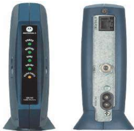
Figure 9-26 A cable modem.
