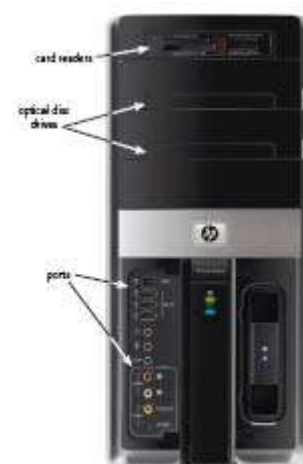
Figure 4-37 External bays usually are located beside or on top of one another.
