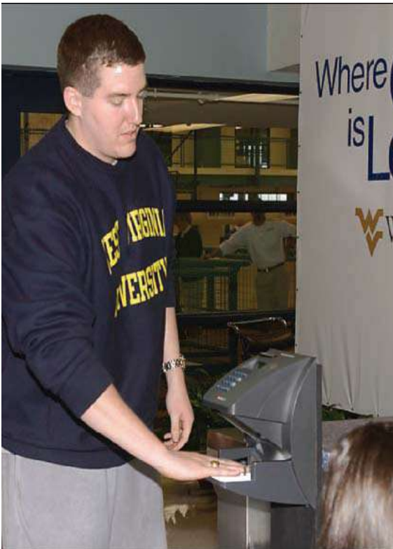
Figure 5-38 A hand geometry system verifies this student's identity before he is allowed access to the school gymnasium.
