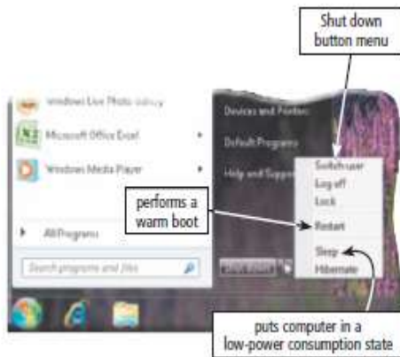
Figure 8-2 To reboot a running computer, click the Shut down button arrow and then click Restart.
