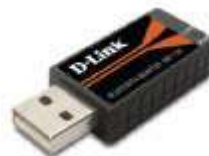
Figure 4-33 A Bluetooth wireless port adapter, such as the one shown here, converts a USB port into a Bluetooth port.
