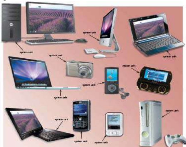
Figure 4-1 All sizes of computers and mobile devices have a system unit.
