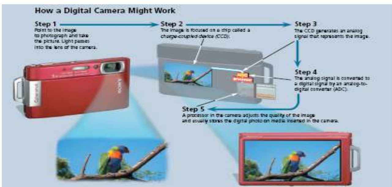
Figure 5-20 This figure shows how a digital camera might work.
