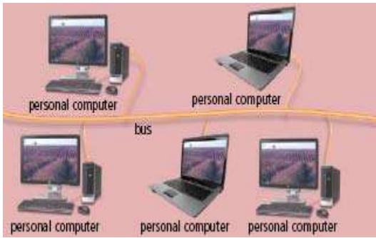
Figure 9-17 Devices in a bus network share a single data path.
