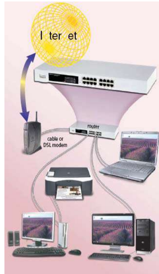
Figure 9-31 Through a router, home and small business networks can share access to a high-speed Internet connection such as through a cable or DSL modem.
