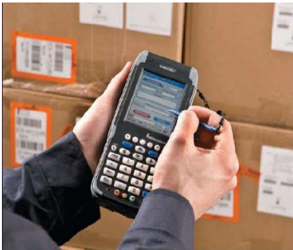
Figure 5-36 A warehouse employee uses this rugged handheld computer, which includes a bar code reader, that wirelessly transmits information about the scanned item to the store's inventory system.
