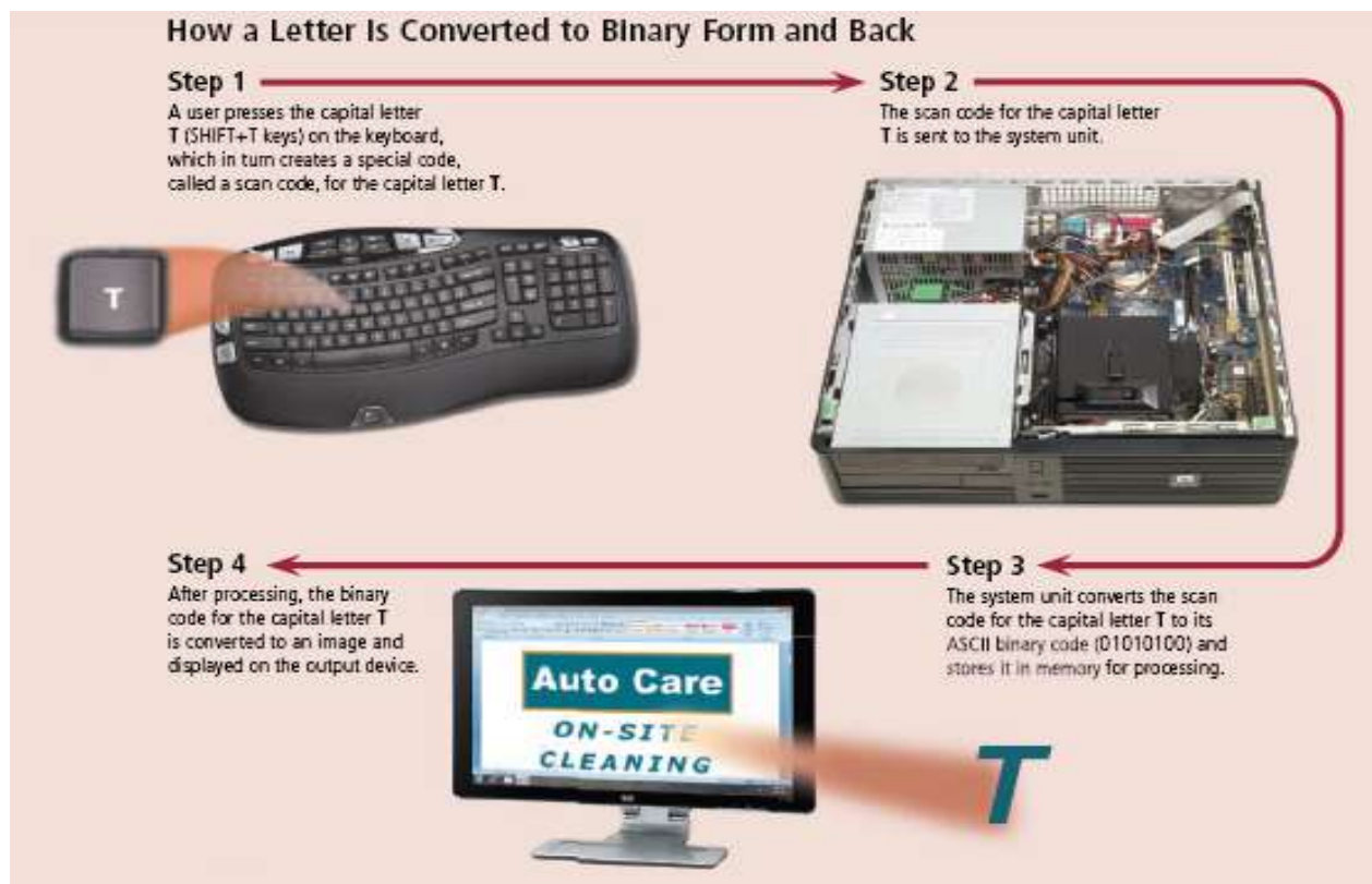
Figure 4-15 This figure shows how a letter is converted to binary form and back.
