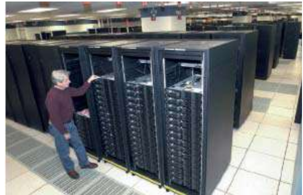
Figure 1-27 This supercomputer, IBM's Roadrunner, can process more than one quadrillion instructions in a single second.
