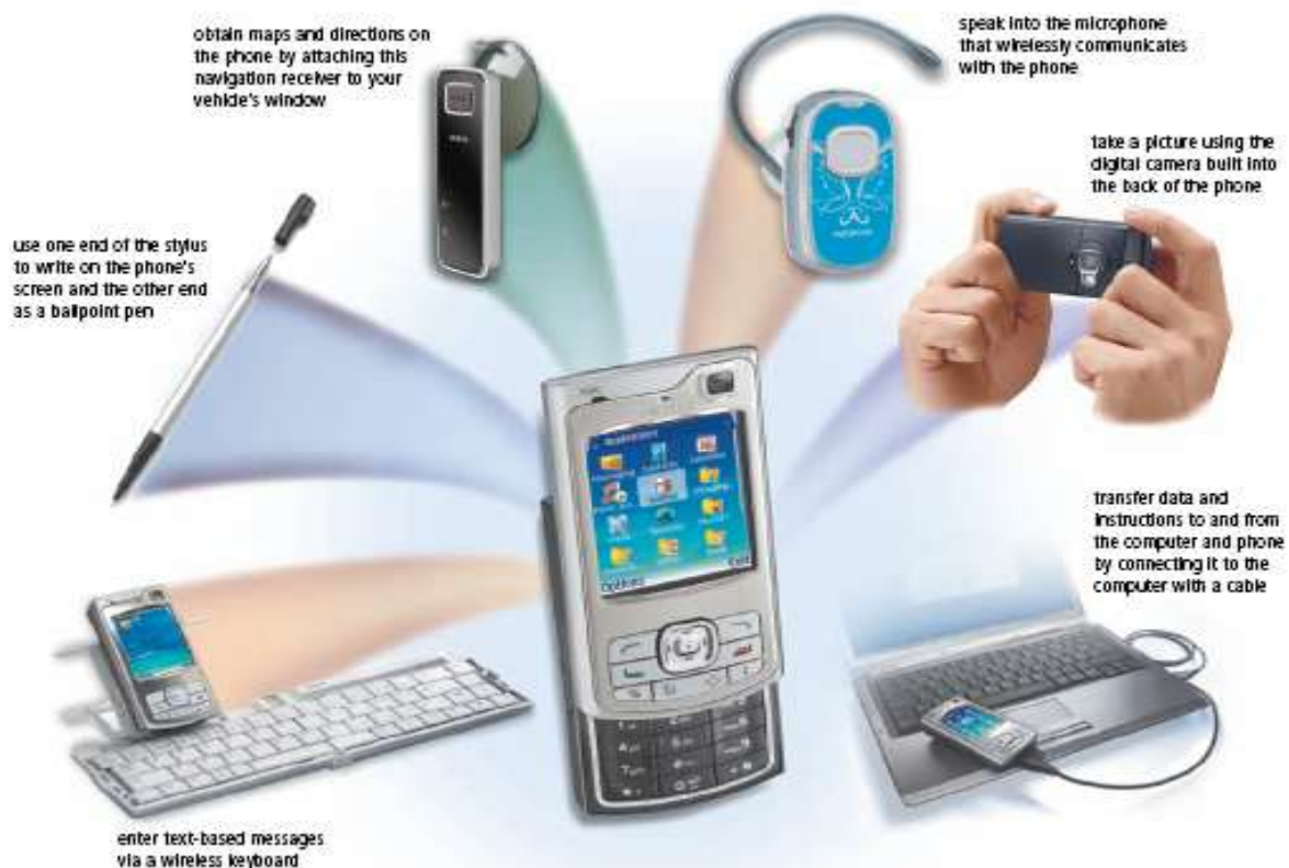
Figure 5-17 Besides a touch screen and basic stylus, users have a variety of other options for entering data and instructions into a smart phone.
