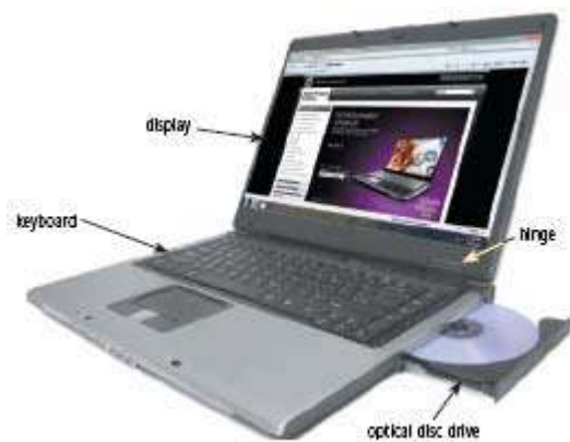
Figure 1-17 On a typical notebook computer, the keyboard is on top of the system unit, and the display attaches to the system unit with hinges.
