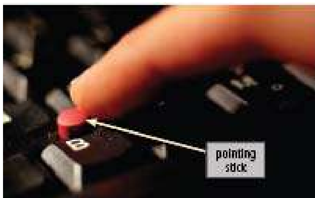
Figure 5-11 Some notebook computers include a pointing stick to allow a user to control the movement of the pointer.
