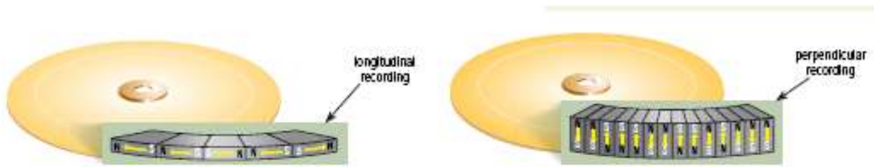
Figure 7-6 Magnetic particles are aligned horizontally in longitudinal recording and vertically in perpendicular recording.
