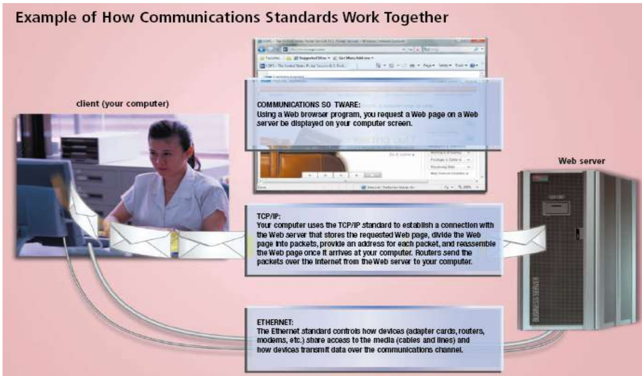
Figure 9-19 Network communications use a variety of standards to ensure that data travels correctly to its destination. Some standards used in Internet communications include the TCP/IP and Ethernet standards, as shown in this figure.
