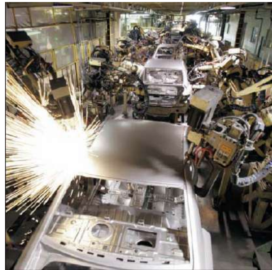
Figure 1-43 Automotive factories use industrial robots to weld car bodies.
