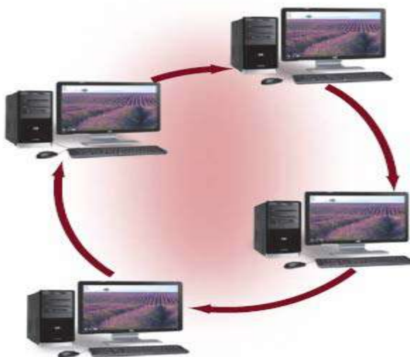
Figure 9-18 On a ring network, all connected devices form a continuous loop.
