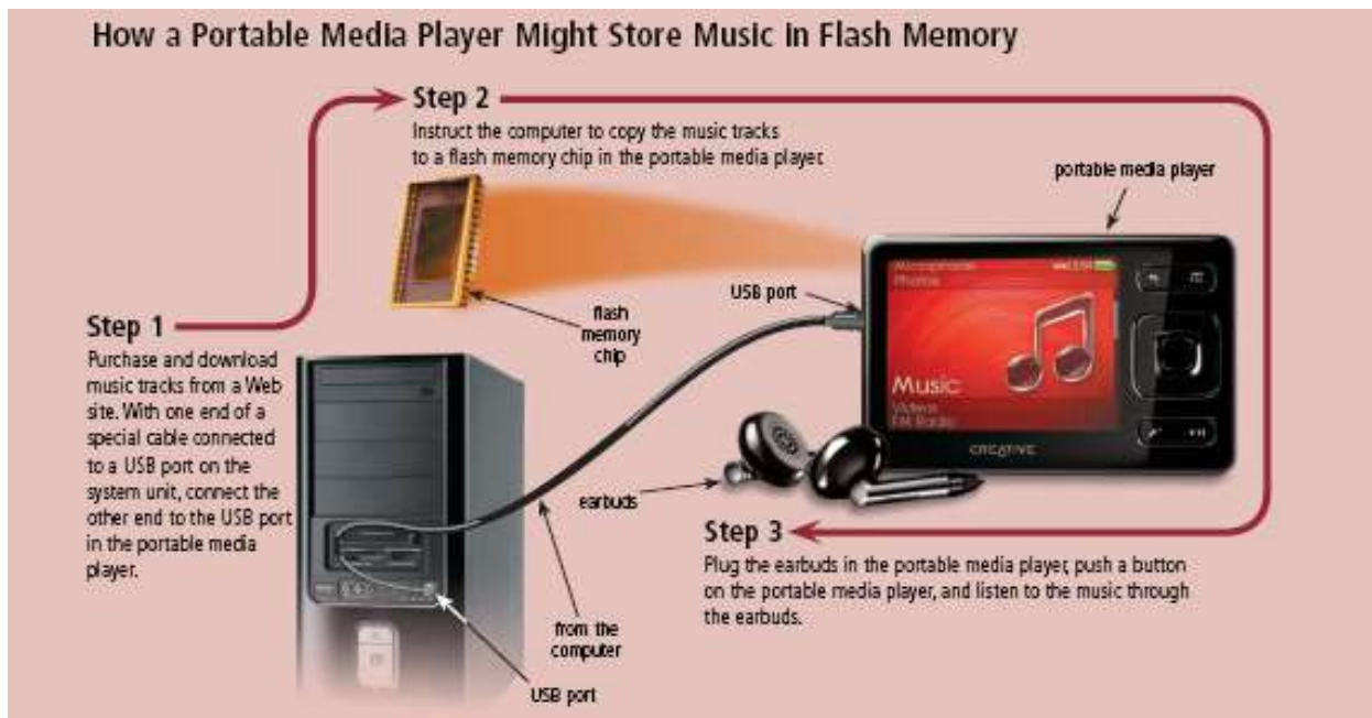
Figure 4-23 This figure shows how a portable media player might store music in flash memory.
