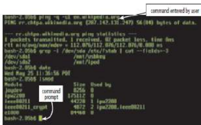
Figure 8-5 A command-line interface requires you enter exact spelling, grammar, and punctuation.
