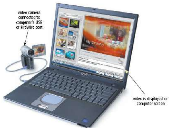
Figure 5-24 Home users can transfer videos to their computers and then use video editing software to edit the video.
