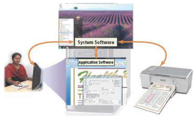
Figure 3-2 A user does not communicate directly with the computer hardware. Instead, system software is the interface between the
