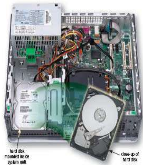
Figure 7-5 The hard disk in a desktop personal computer is enclosed inside an airtight, sealed case inside the system unit. (In this and other hard disk photos in the book, the top plate is removed from the hard disk for illustration purposes.)
