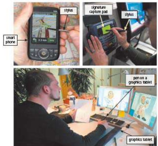
Figure 5-16 You use a stylus or a pen to write, draw, or make selections on a screen, signature capture pad, or graphics tablet
