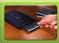
A **removable hard disk** is a hard disk that you insert and remove from a drive
