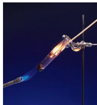
Heating potassium chlorate produces oxygen, which supports the combustion of wood splint.
