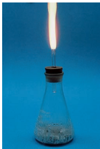
The reaction of calcium carbide with water produces acetylene, a flammable gas.
