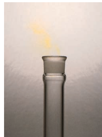
N_2O_5 decomposes to give NO_2 (brown color) and colorless O_2 gases.
