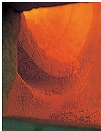
Figure 18.7 The production of CaO from CaCO 3 in a rotary kiln.
