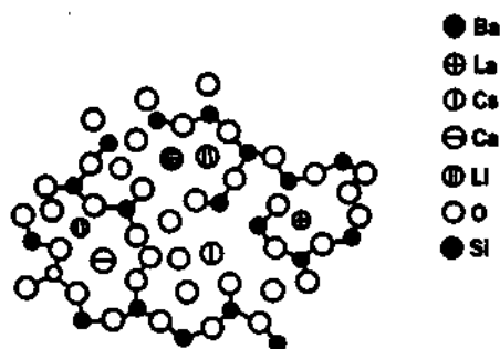
Fig. 9-9. The structure of glass used in glass electrodes. (After G. E. Perley, Anal. Chem. 21, 392, 1949).
