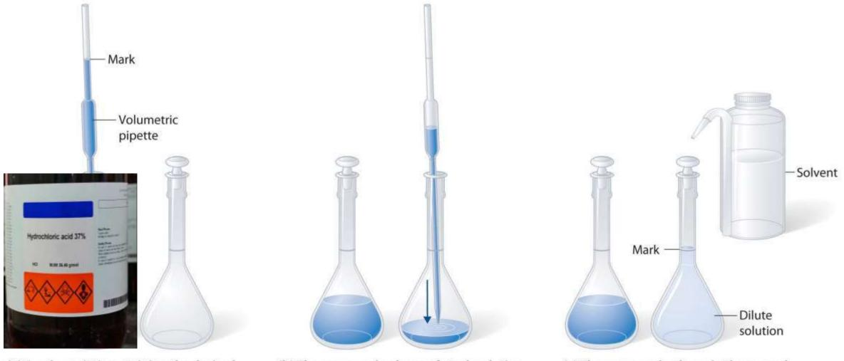
(a) A volume ( $V_s$ ) containing the desired moles of solute ( $M_s$ ) is measured from a stock solution of known concentration.
