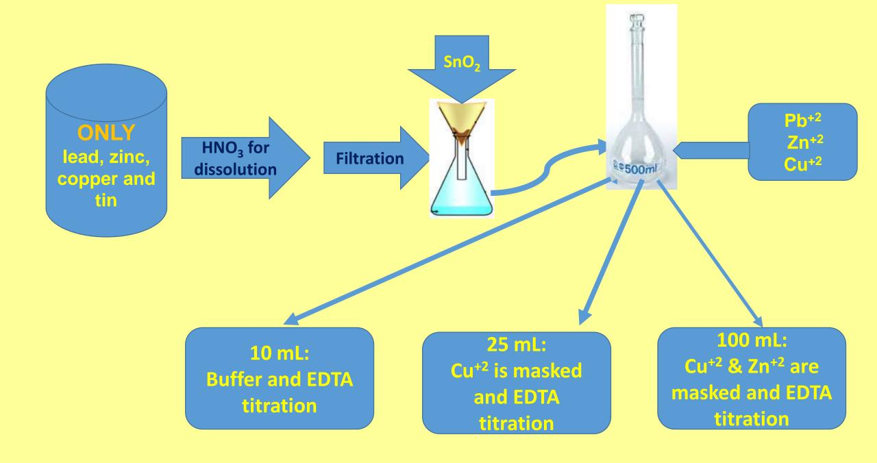
10 ml no mmol EDTA = 37.5 (ml)\*0.0025 (M)= 0.09375 (mmol) = no mmol( Zn + Cu + Pb) = 0.09375 (mmol)
