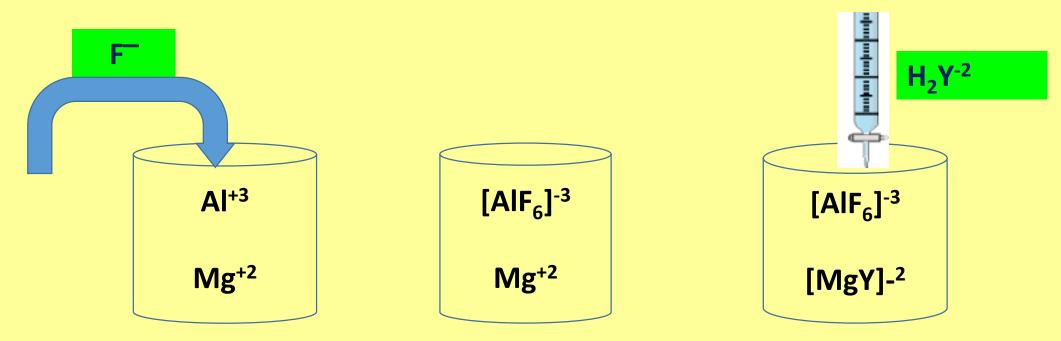
Flouride ion is a masking agent for Al<sup>+3</sup>, which will not interfere with EDTA titration.
