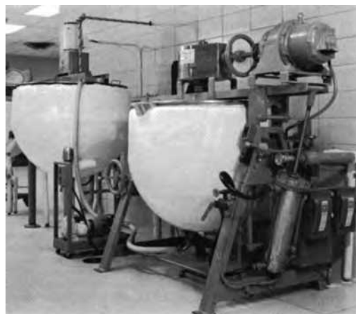
FIGURE 12.3 Large heated tanks for preparation of the melt in commercial production of suppositories by molding. (Courtesy of Wyeth-Ayerst Laboratories.)
