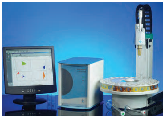
FIGURE 4.4 Electronic tongue to assist in formulation development. (Courtesy of Alpha MOS.)
