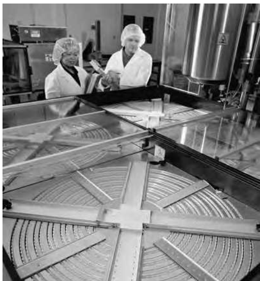
FIGURE 12.4 Highly automated large-scale production of molded suppositories prepared and packaged in strips. (Courtesy of Paddock Laboratories.)
