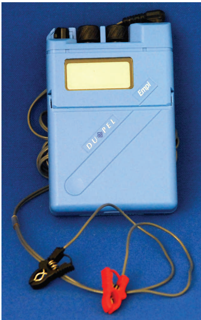
FIGURE 20.1 The DuPel iontophoresis system showing the connections to which a passive and an active (drug-containing) electrode will be attached.
