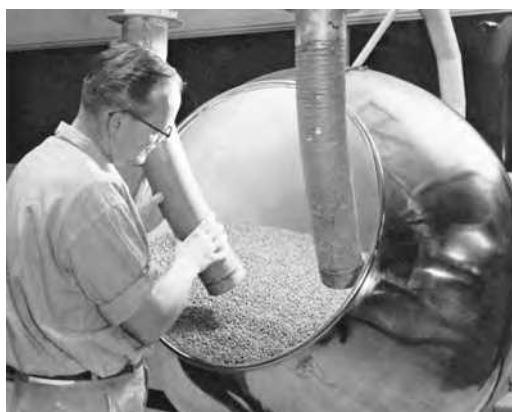
FIGURE 8.30 Tablet coating, an old-style coating pan, showing the warm air supply and the exhaust. (Courtesy of Wyeth Laboratories.)
