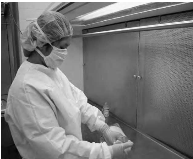
FIGURE 15.22 Hyperalimentation being prepared in a horizontal laminar flow hood. (Courtesy of Ms Amy Schuppert Smith.)
