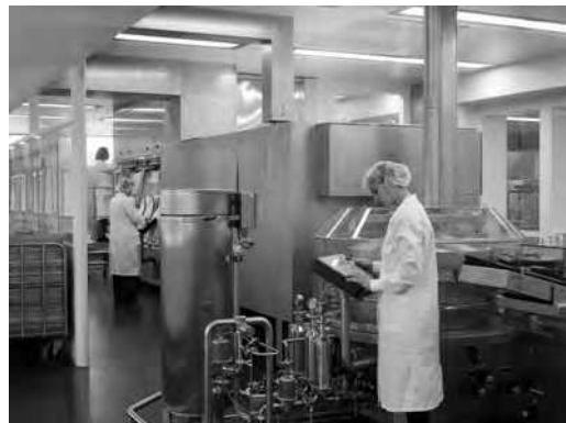
FIGURE 15.21 Filling and sealing of ampuls/vials (nonfreeze-dried preparations). (Reproduced with permission of Schering Corporation. All rights reserved.)
