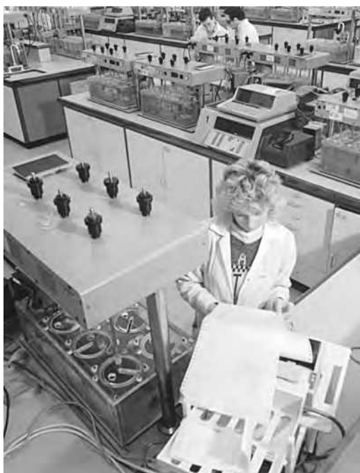
FIGURE 8.17 A modern computer laboratory dedicated to studies of drug dissolution from solid dosage forms. Included are Erweka dissolution baths, Hewlett-Packard computers, and Hewlett-Packard diode assay spectrophotometers. (Courtesy of Elan Corporation, plc.)
