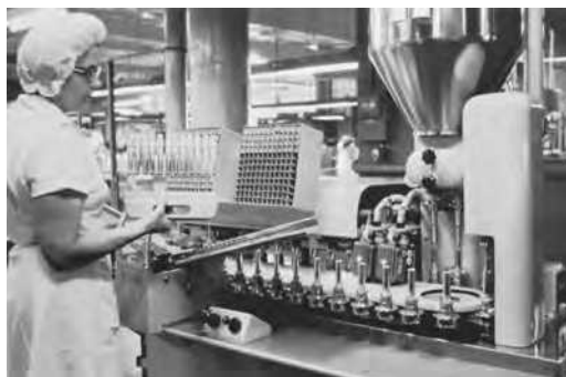
FIGURE 10.6 Arenco tube-filling machine automatically fills 125 tubes a minute with the proper amount, tightens the cap, orients each tube by electric eye so that the label faces forward, then closes and crimps the end. (Courtesy of Eli Lilly and Company.)
