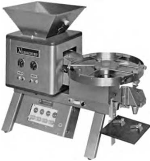
FIGURE 7.19 Versacount Model automatic tablet and capsule counting and filling apparatus. (Courtesy of Production Equipment Co.)
