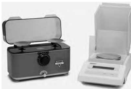
FIGURE C.3 Prescription balances: Torbal torsion balance ( left ) and Ohaus electronic balance. (Courtesy of Total Pharmacy Supply.)
