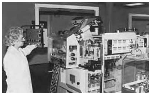
FIGURE 11.10 Equipment used in cutting and packaging transdermal drug delivery patches. (Courtesy of Schering Laboratories.)
