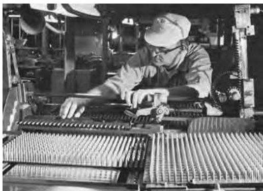
FIGURE 7.2 Body of capsules and their caps are shown as they move through an automated capsule-making machine. Each machine is capable of producing 30,000 capsules per hour. It takes a 40-minute cycle to produce a capsule. (Courtesy of SmithKline Beecham.)
