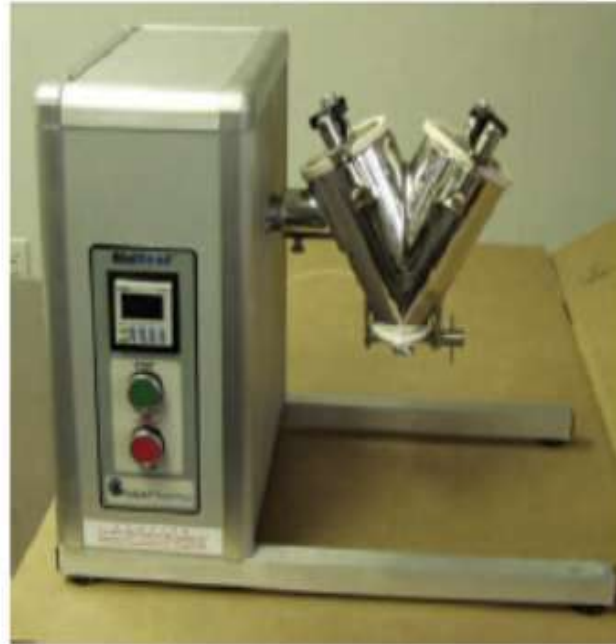
FIGURE 6.4 Laboratory-scale V-blender. (Courtesy of GlobePharma.)
