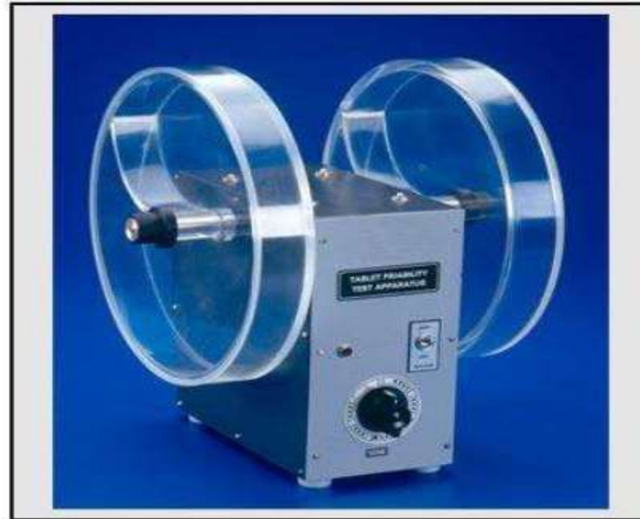
Fig-5: Friability apparatus
