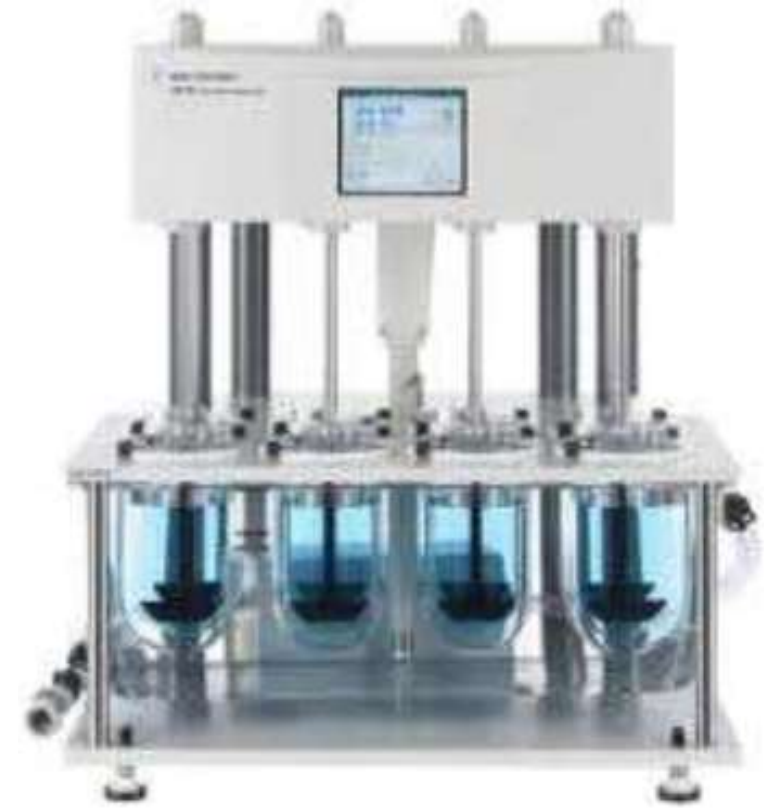
Fig-9: Dissolution apparatus paddle type
