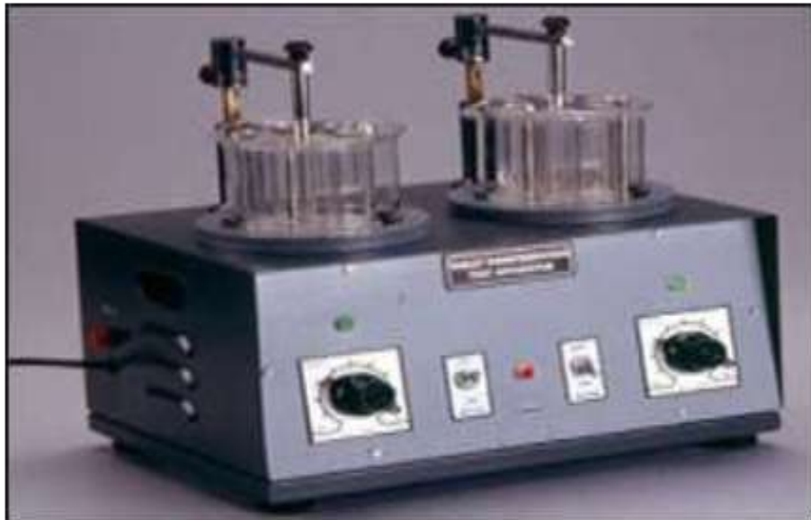
Fig-6: Disintegration apparatus
