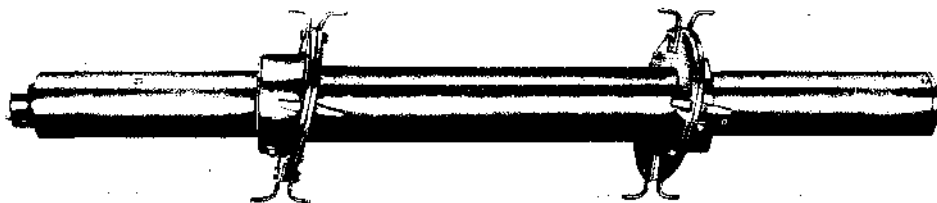
FIG. 23-4. Liquid-dispersion bar increases or "intensifies" speed and thoroughness of liquid-solid blends. (Courtesy of Patterson-Kelley, Co., Division of Harsco Corp.)
