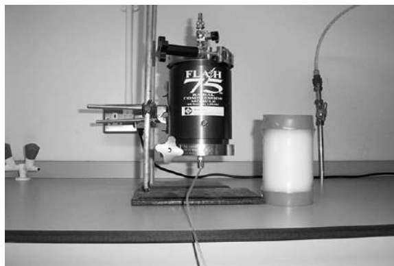
Fig. 7.3 Biotage flash chromatograph. Fast separations are achieved with good resolution.
