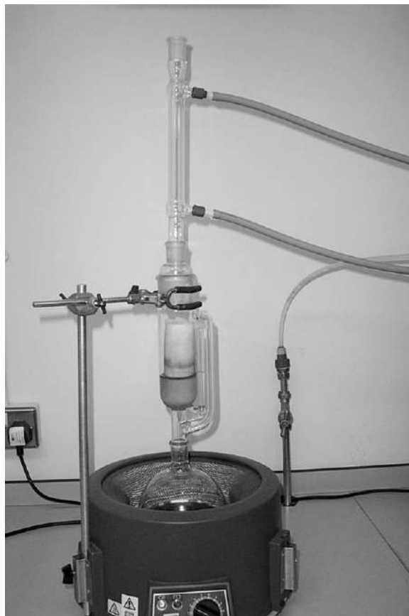
Fig. 7.1 Soxhlet extraction apparatus. Generally used to give greatest yield of extract when extracts are stable in hot solvent.
